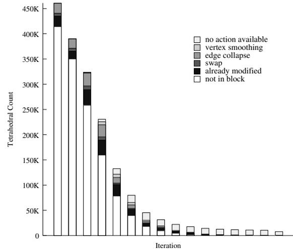
**Figure 4:** Each bar in this visualization represents an iteration of the algorithm. The height of the bar is the number of tetrahedra at the beginning of the iteration, with the poorest tetrahedra at the top, where early computation is focused. The number of elements is quickly reduced and then levels off to allow the model to settle into the best compromise between element quality and surface detail for the desired number of tetrahedra.
