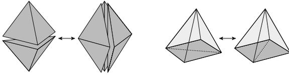
**Figure 5:** Two tetrahedra that share a face may be replaced with three tetrahedra that share an edge (or vice versa). Similarly, two tetrahedra that share a face and have neighboring boundary faces that are nearly parallel can be replaced with two tetrahedra that essentially swap the edge between these two boundary faces. Illustration redrawn from [16].
