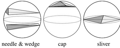
**Figure 1:** Illustration of poorly-shaped tetrahedral elements. Unlike the 2D case, it is not sufficient to judge element shape quality by the ratio of shortest and longest element edges. While this test detects needle and wedge tetrahedra, it fails for sliver tetrahedra. A better metric in 3D is the minimum solid angle. Illustration redrawn from [41].
