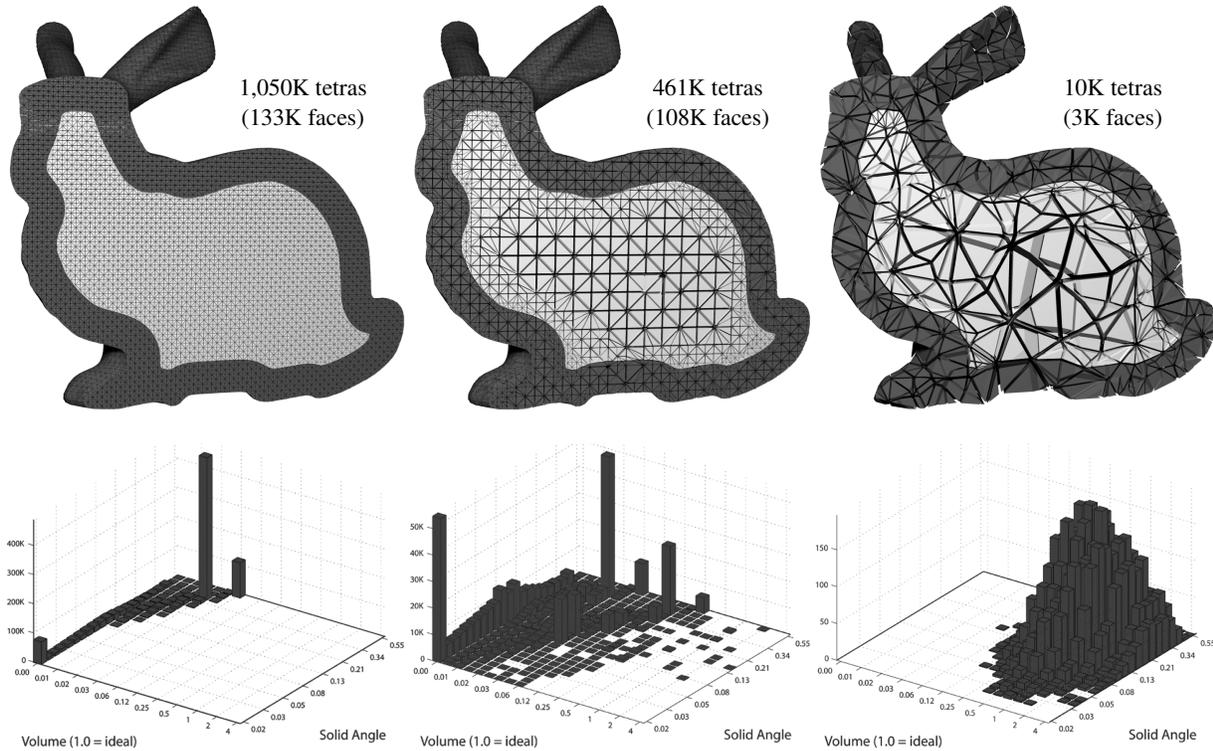
**Figure 2:** The meshes generated from a uniform distance field (top left) and an octree version of the same distance field (top middle) have similar boundary quality. The simplified version (top right) maintains the exterior and interior interfaces. Below each mesh is a histogram of the element quality. The leftmost corner of each plot represents the worst quality elements (near zero volume, near zero minimum solid angle), and the rightmost corner represents the best elements.
