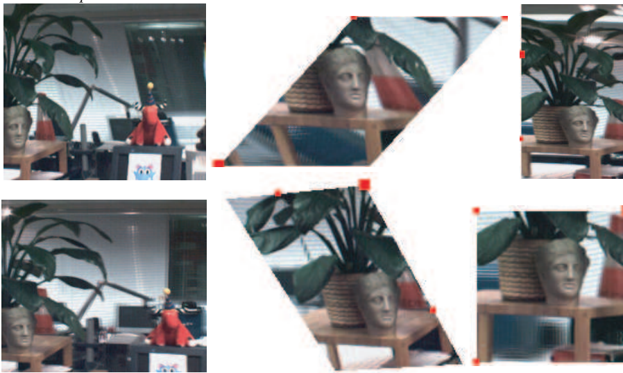
FIG. 6. GLC images synthesized from a 3D light field: (a) is a pushbroom panorama, (b) is a cross-slit panorama.
