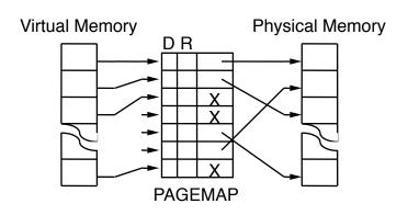
Several programs may be simultaneously loaded into main memory, each in its separate context:
