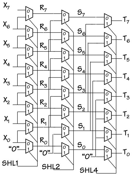
If we connect our "shift-left -two" shifter to the output of our "shift-left-one" we can shift by 0, 1, 2, or 3 bits.
