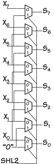
Using the same basic idea we can build left shifters of arbitrary sizes using muxes.
