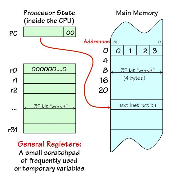
In Comp 411 we'll use a clean and sufficient subset of the MIPS-32 core Instruction set.
