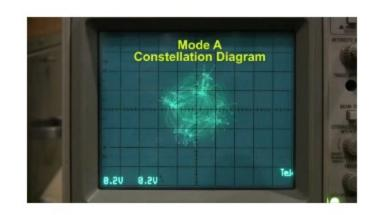
A simple binary coding does not make good use of the dynamic range of a digital signal, however, if you put the codes too close noise becomes a problem.
