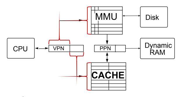
OBSERVATION: If cache line selection is based on unmapped page offset bits, RAM access in a physical cache can overlap page map access. Tag from cache is compared with physical page number from MMU.
