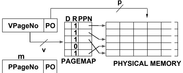
(v + p) bits in virtual address (m + p) bits in physical address 2<sup>v</sup> number of VIRTUAL pages 2<sup>m</sup> number of PHYSICAL pages 2<sup>p</sup> bytes per physical page 2<sup>v+p</sup> bytes in virtual memory 2<sup>m+p</sup>bytes in physical memory (m+2)2<sup>v</sup> bits in the page map Typical page size: 4K – 128K bytes Typical (v+p): 32 or 48 or 64 bits Typical (m+p): 30 – 39 bits (1GB – 512 GB)
