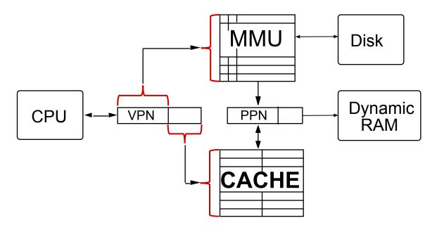
OBSERVATION: If cache line selection is based on unmapped page offset bits, RAM access in a physical cache can overlap page map access. Tag from cache is compared with physical page number from MMU.
