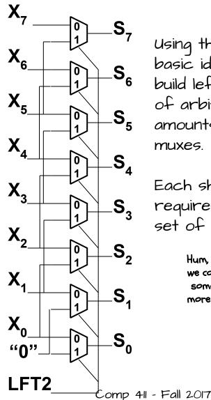
Using the same basic idea we can build left shifters of arbitrary shift amounts using muxes.
